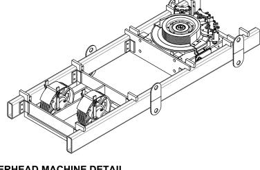
OVERHEAD MACHINE DETAIL FOR REFERENCE ONLY CAPACITY - UP TO 3,500 LBS SPEED - UP TO 350 FPM
